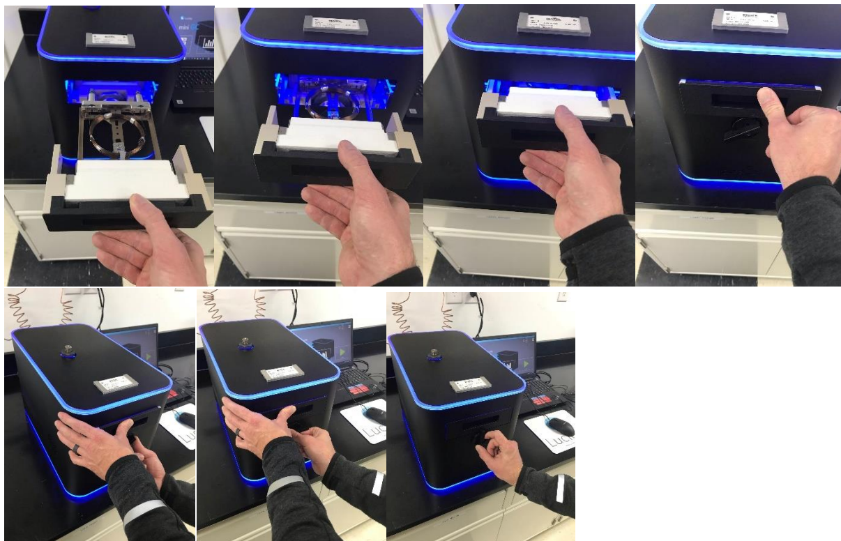
Putting the Column Caddy with Column Holder and column into the miniGC
