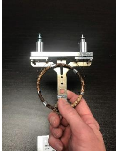
1. Preinstalled column: column in Column Holder
