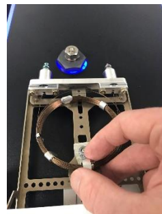
4. Column Holder being placed on Column Caddy via 2 alignment pins
