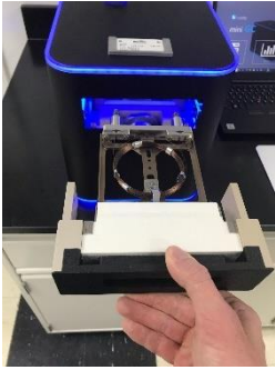
5. Column Caddy being inserted into miniGC with Column Holder in place
