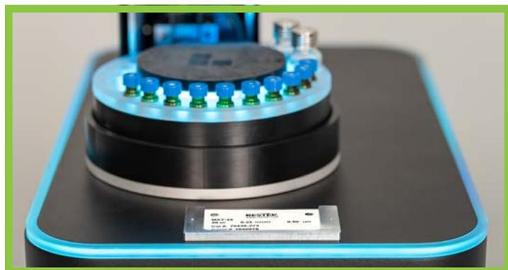
Organize your lab with the Column Storage Rack that allows users to store columns that are not in use in a convenient rack that saves space and seals the ends of the columns to prevent contamination.
