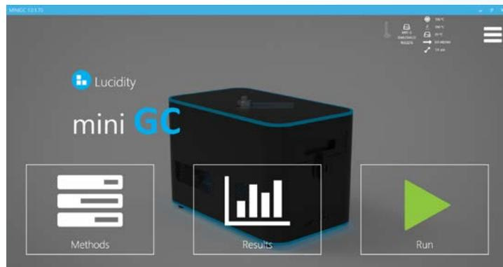
Upon entering the run screen, you are able to create a sequence or set up a single sample. After choosing a run name and a method, the user sees the status of the run parameters as they approach the method starting set-points. Once the set-points have been reached, the user can start the run.
