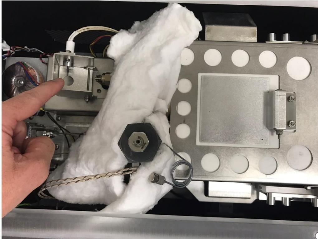
Now you can see inside the unit. These two pictures show the Ignitor Housing. The ignitor housing should normally be in the closed position so that the ignitor is positioned just after the outlet and can ignite the flame in the FID. The Ignitor Housing can be opened as shown in the bottom picture to examine the ignitor.
