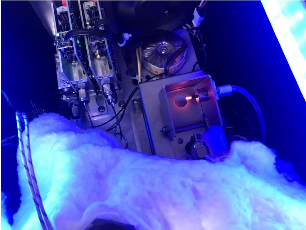
After a few seconds the ignitor should begin to glow as shown in these pictures, which it should do for a few seconds and then go out.
