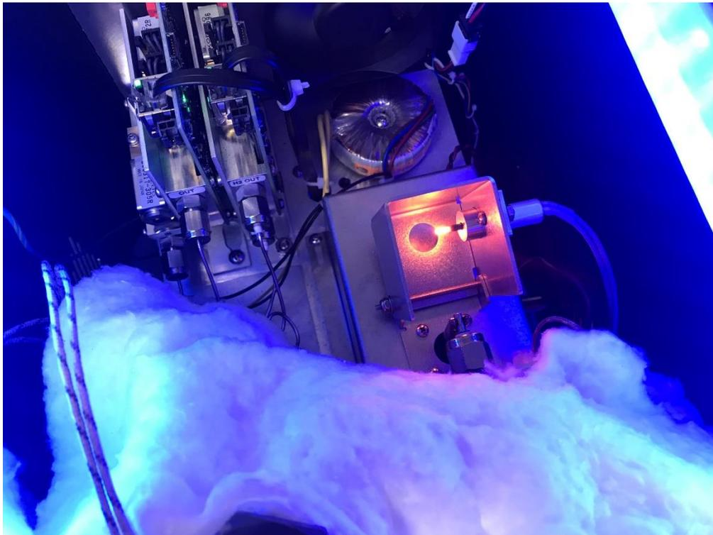
If the ignitor does not glow after pressing ignite then there is a problem with the ignitor itself. It may be unplugged from the board or it may just be bad. If the ignitor does glow after pressing Ignite then the ignitor is okay.
