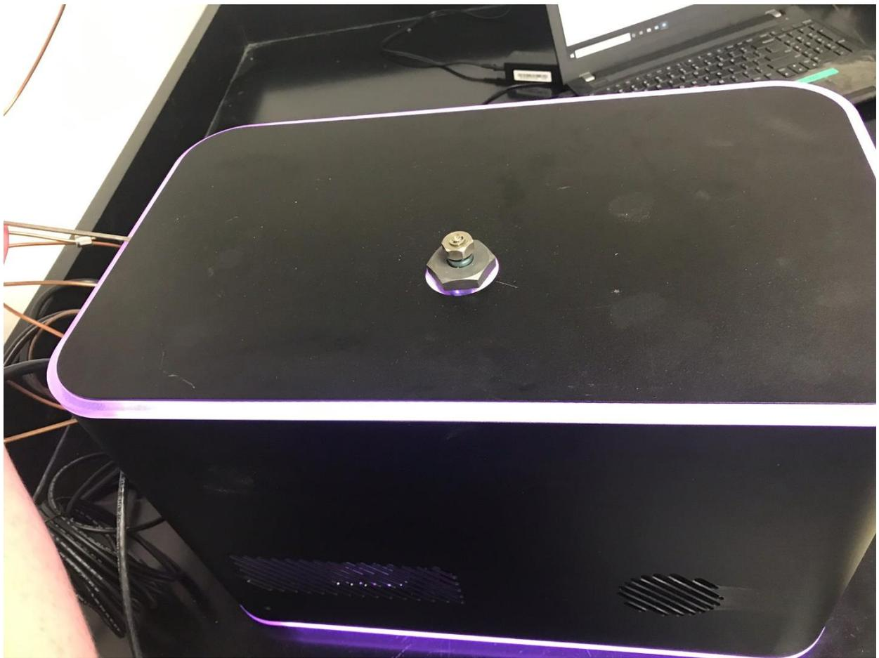
Start by prying up the back of the top cover of the miniGC with a flat blade screwdriver or pair of tweezers. The top plate is only attached to the unit by magnets so by prying it up using the slot in the back you can pull it off of the unit.
